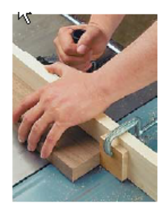
▲ To make repeat cuts, clamp a stop block to the fence.
