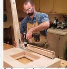
7. Screw the leg hinges to the bottom of the router table top. The legs should bypass each other when they're folded.
