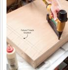
2. Pin the top and bottom skins to the torsion box so they don't shift during clamping. Avoid the T-track locations so you don't rout into a brad later. It only takes a few brads to hold the parts in place.
