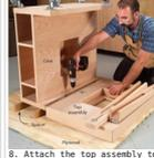
8. Attach the top assembly to the case using a continuous hinge. Use a pair of 2-1/4" spacers under the case to make it level with the top.
