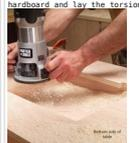
4. Flush-trim the cavity in the bottom of the torsion box assembly. Use a jigsaw to remove most of the waste first.
