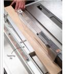
6. Taper the sides of the legs using a taper jig on the tablesaw. The leg sides must be cut to final length before you taper them.
