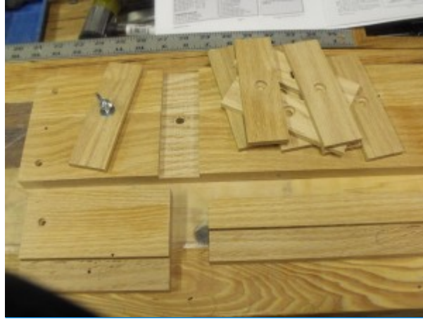
Backer boards. $3.59 1-1/2" x 48" cut to 5" chunk and mount hole drilled
