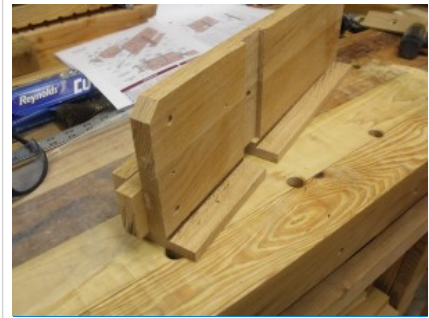
Dry fit both movable and non-movable fence setting on base.
