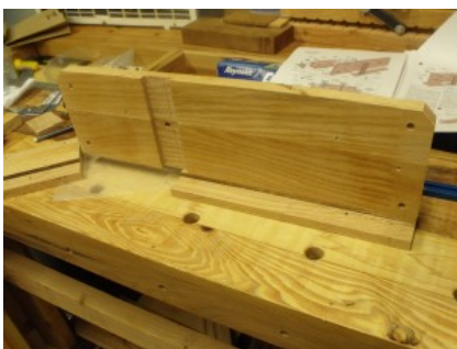
Dry fit Fence setting on base.
