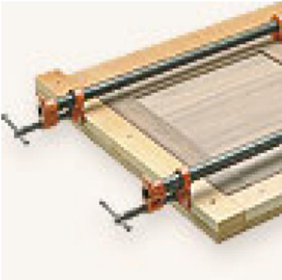
Gluing up a frame and panel door so it ends up perfectly square can be difficult. The pieces always seem to slip out of square during glue-up.
